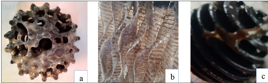
Fig. 12. Biofilm attachment on biofilter growth media, (a) bio ball serrations, (b) wasp nest, (c) bio ball golf
